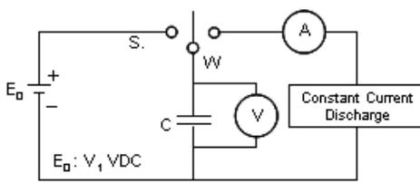
$C = A(\text{Ampere}) \times T \text{ sec} / (V_1 - V_2) \text{V [F]}$
