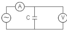
$R[\Omega] = V[V] / I[A] \quad * i[\text{mA}] = I[A] \times 10^{-3}$ <p>R : Internal resistance(ESR) [<math>\Omega</math>]<br/> V : Measured voltage between terminals [V]<br/> i : Current 1mA(A.C.)</p> $\text{ESR}[\Omega] = V / i$                                                                                                                                                |
